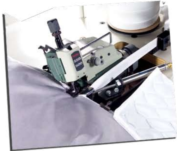
5a With the SSB-500, single-sided bed binder, non-skid panels are flanged and taped to the border in one easy step. The SSB-500 prepares the non-quilted side of the no-flip bedding and eliminates pre-flanging on the non-skid panel. The high-lift walking foot sewing head accepts either border rolls or pre-closed borders. (Eliminates one tape edge operation.)
