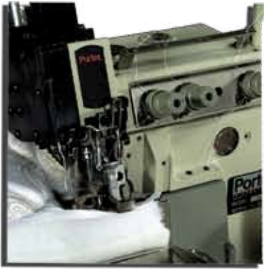
4 PFM-515 high-speed flanger used for attaching flange to the border material.
