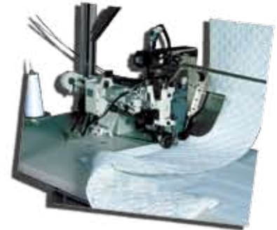
5b Depending on the desired look, an alternative to 5a would be to utilize the same GPT-1000AP to create a tapeless one-sided mattress. (Example: reversing the continental foundation cover process as the underside of the bed)
