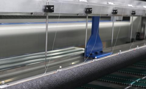
The Gribetz<sup>®</sup> XT9<sup>™</sup> sews layers of foam and other comfort materials together instead of gluing – completing the process in a single 35-second pass and reducing costs by 95%. It automatically detects material stack size, and a set of nine needles stitches all the layers at once.
