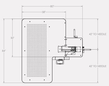
A powerful air table makes it easy to turn heavy goods throughout the binding process. The working surface can be electronically raised or lowered 12" (30.5 cm) to fit the personal comfort of any employee at the touch of a button.
